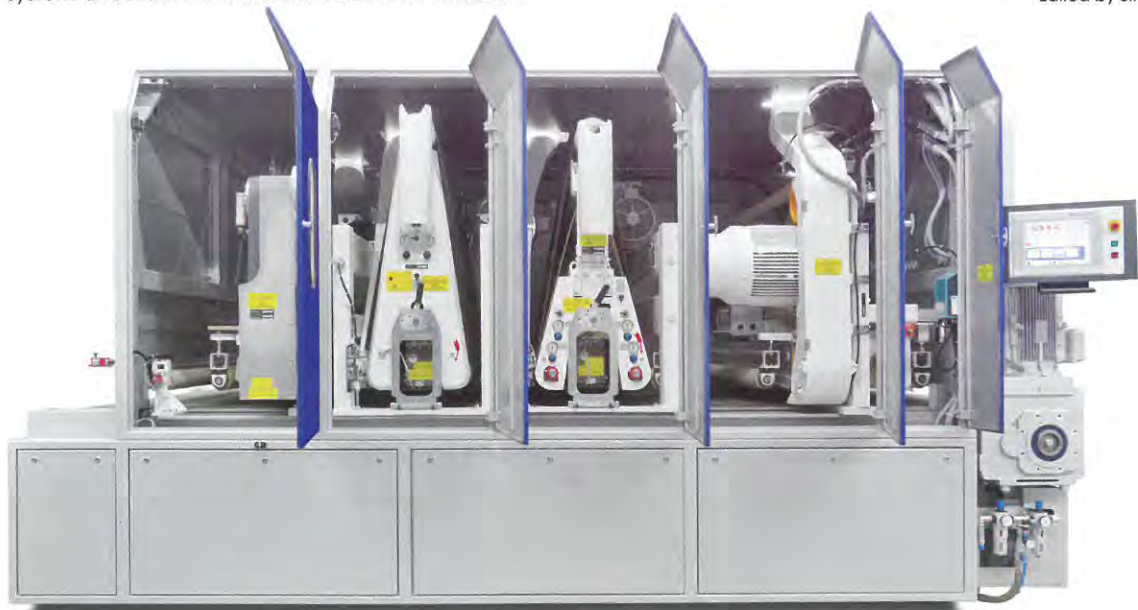
A Heesemann KSA 8 sanding machine equipped with four sanding units
